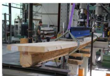
Fig. 11 4-point bending test source: Meyer
