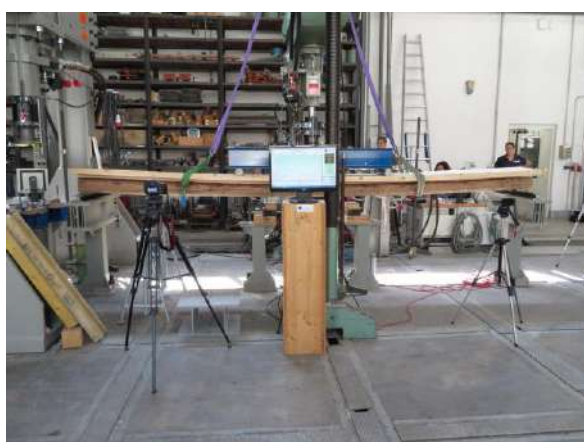
Fig. 12 4-point bending test on the test beam source: Jäger
