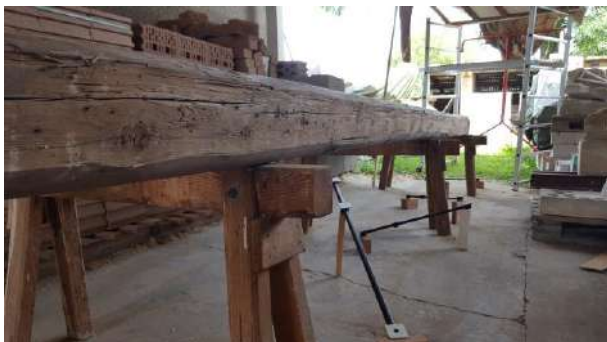
Fig. 8 Reference standards (black bars with measurement points) for optimizing the SfM method source: Meyer
