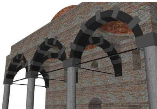
Fig 14. Strengthening of the brick masonry arches by externally bonded CFRP
