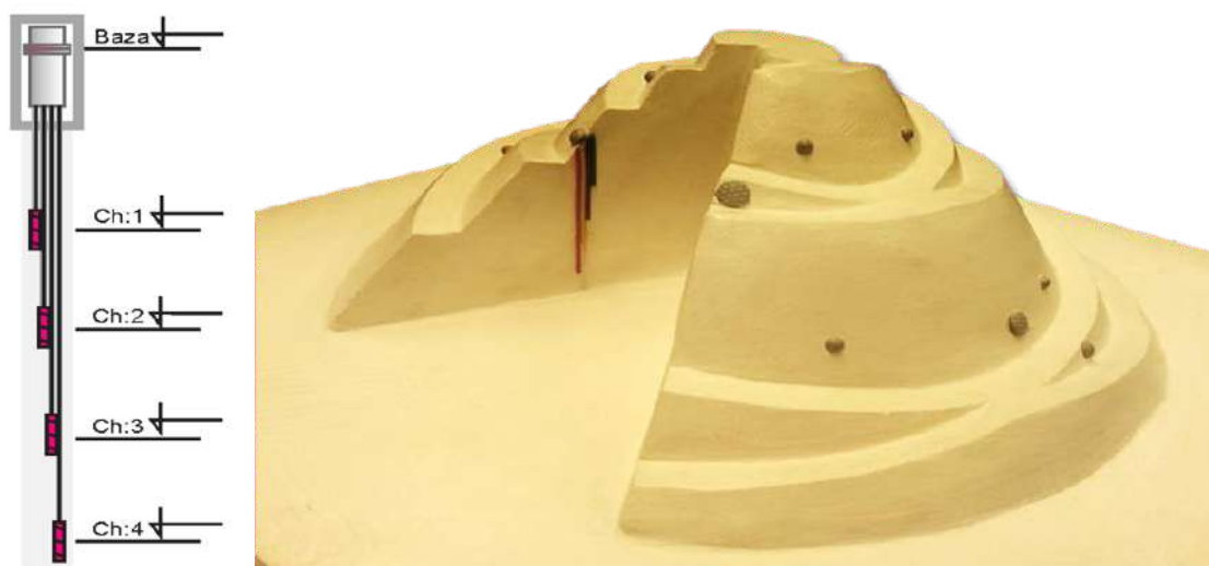
Fig. 5. Details of vertical displacement measurements.
