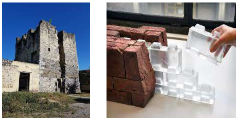
Fig. 19. Cast glass elements proposed for the restoration of Lichtenberg Castle, Maastricht https://commons.wikimedia.org/wiki/File:2016_Maastricht_St-Pietersberg_Lichtenberg
