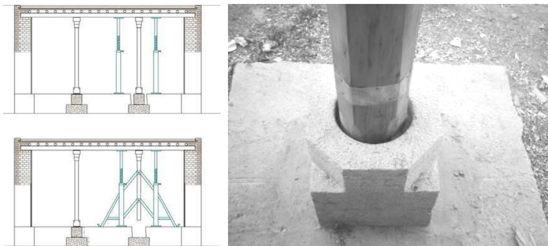
Fig. 24a: Collapsing the decayed foundation and restoration of the foundation
