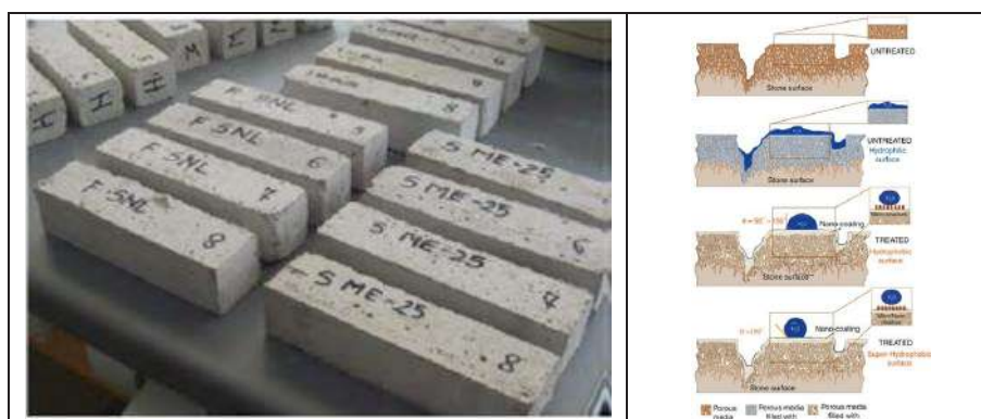
Fig. 3. Condition of the plaster samples after examination on resistance to salt crystallization
