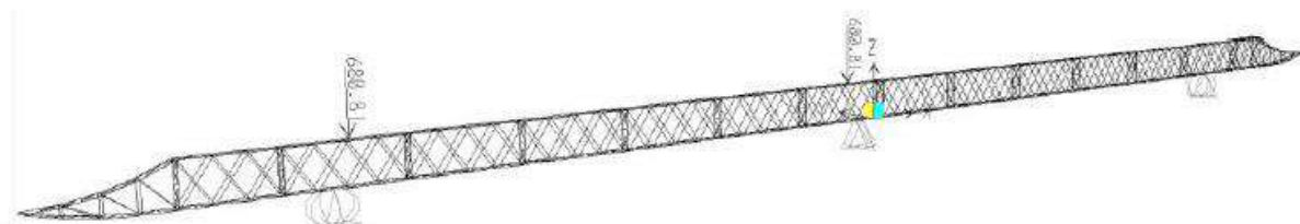
Fig.10i. Support conditions and loads arrangement for scheme SH 2.1. ( F=680.81\text{kN} ).
